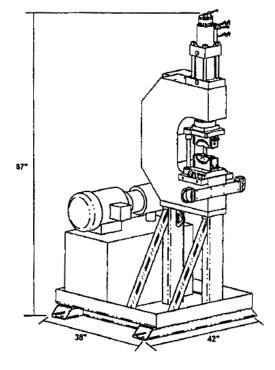
• Double-cavity crimp die contains both a left and right crimping stations.
