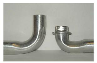
Taking a tube with a 90° bend close to the end, the **M04-VH-8**, *Vertical Bump Machine*, with capacity of 8 strokes, flattens the radius of the tube and completes the end form, creating a lower overall profile.
