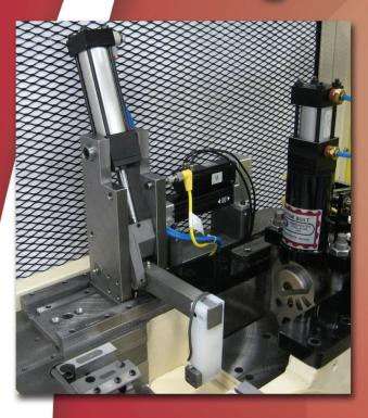
Our servo positioning flag stop system helps to quickly adjust tube out through the machine's H.M.I. (human machine interface). It provides consistent adjustments for quicker setup up times.
