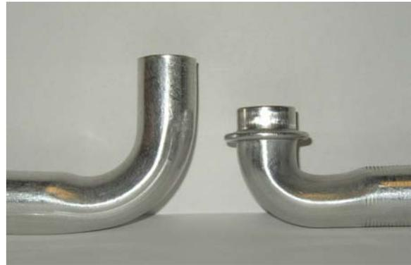
Taking a tube with a 90° bend close to the end, the **M04-VH-8**, *Vertical Bump Machine*, with capacity of 8 strokes, flattens the radius of the tube and completes the end form, creating a lower overall profile.
